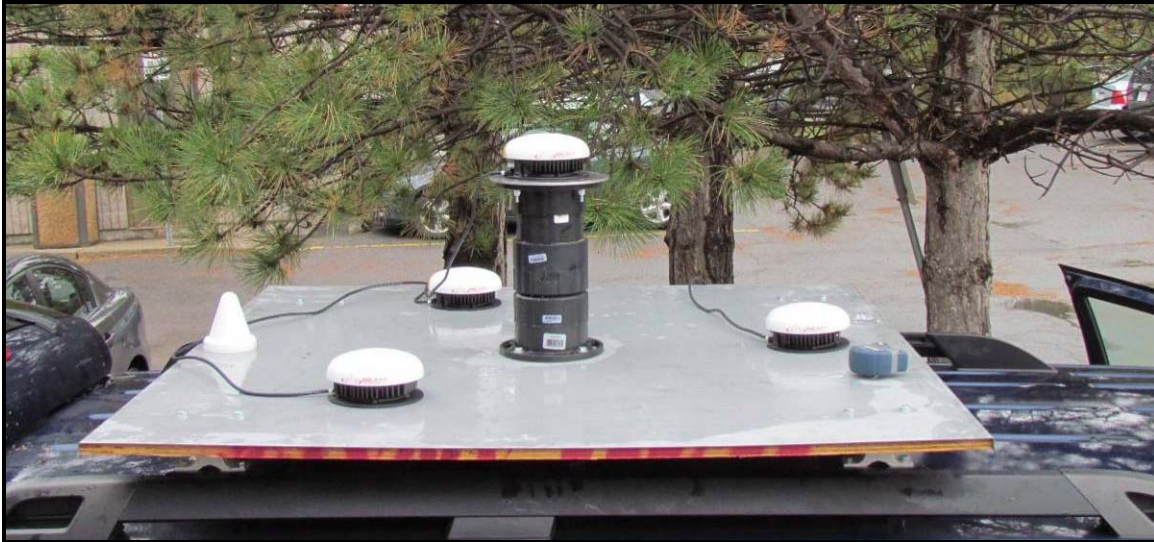
Figure 5. Antenna installation on vehicle.
