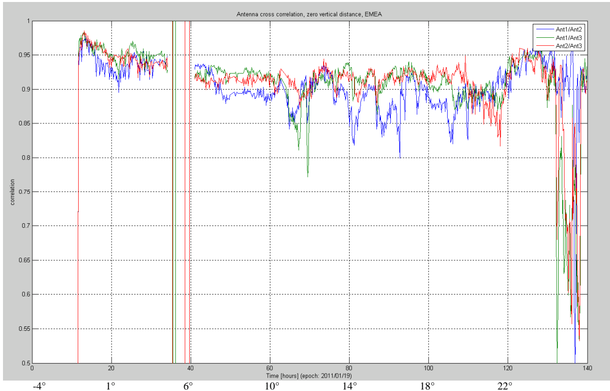
Figure 10. Power cross-correlation, horizontal separation (EMEA CW, eastbound crossing).
